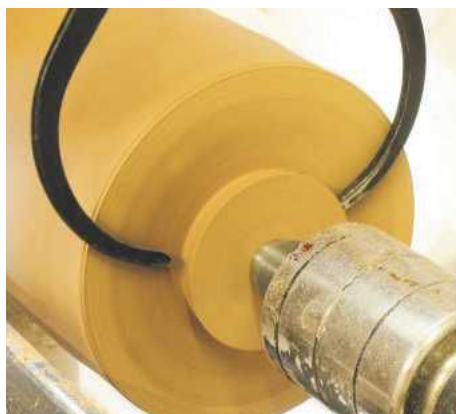
▲ Pic.2 If you are using dovetail jaws it is important to get the spigot the right size. Bow-leg callipers are perfect as the leg ends have been rounded over to stop them digging into the wood
